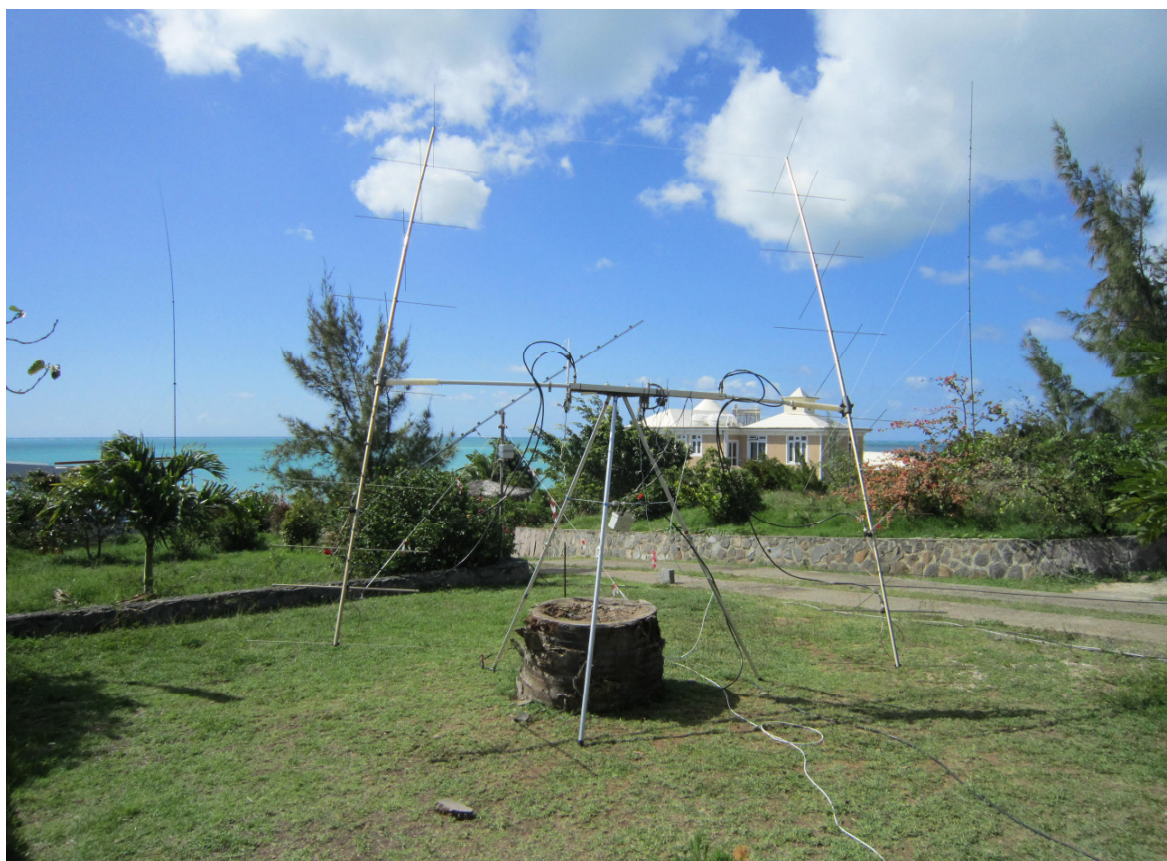
The 2m EME setup at 3B9EME: a 2 x 8 ele XPOL
